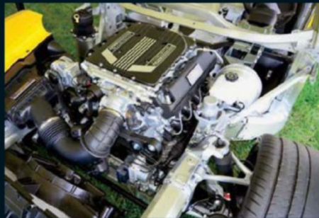
Chevrolet displayed this cutaway of the '15 Z06 that gave us a chance to inspect the awesome 650hp LT4. This compact engine packs a lot of punch. Notice the 625hp signs on the valve covers have not been updated.
