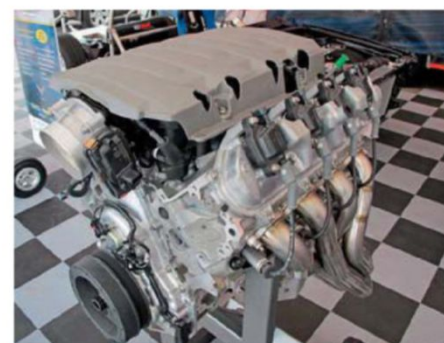
Scoggin-Dickey was on hand with a slew of cool Chevrolet Performance crate engines on display. The newest offering was this Gen 5 LT1. It displaces 6.2 liters and features direct injection, active fuel management, and variable valve timing. Output is rated at 460 hp and 465 lb-ft of torque.
